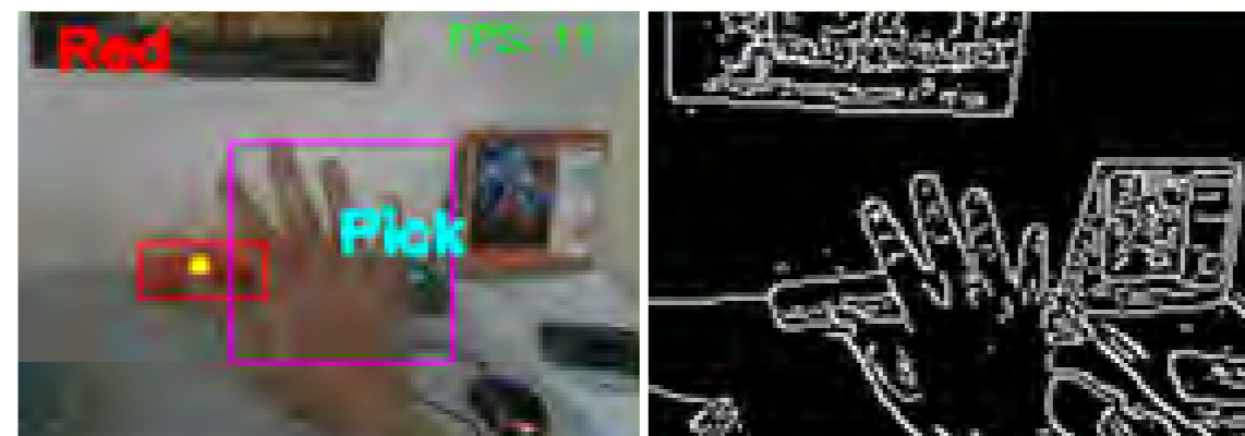
If the hand and object regions overlap, the system will issue 'pick up' for the visually impaired to grab the object
