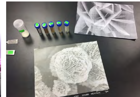
(Inset photos) Three-dimensional hierarchical structure photocatalysts with flower-like and spherical-like morphologies. The different tubes also show the colour changes of palm oil mill effluent for different exposure times under photocatalytic reaction.
