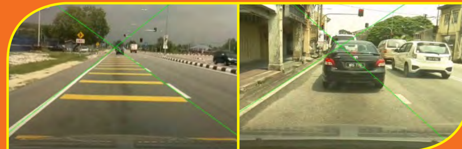
Lane Detection Output: Two-lane roadway
