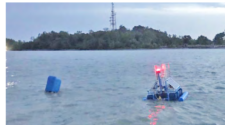
▲ The IoT Detachable Waterway Monitoring Device being tested at the Kuala Selangor River for 1 week
